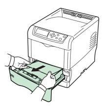
2 While pulling the green paper transfer unit release lever, pull out the paper transfer unit.
